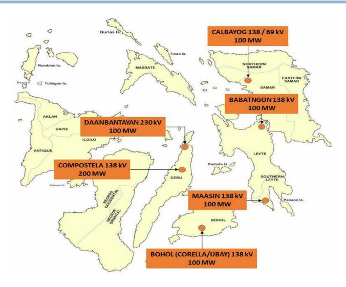
Note: Ideal Location of Power Plants without the need for any significant transmission reinforcement.
