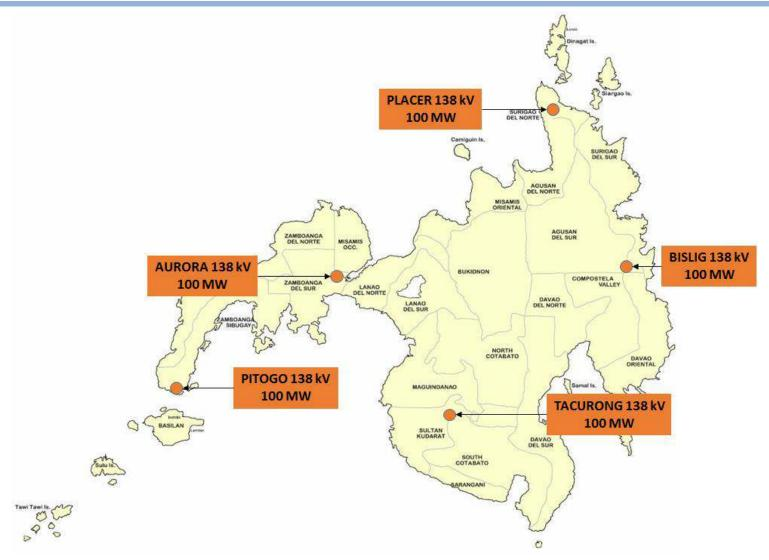
Note: Ideal Location of Power Plants without the need for any significant transmission reinforcement.
