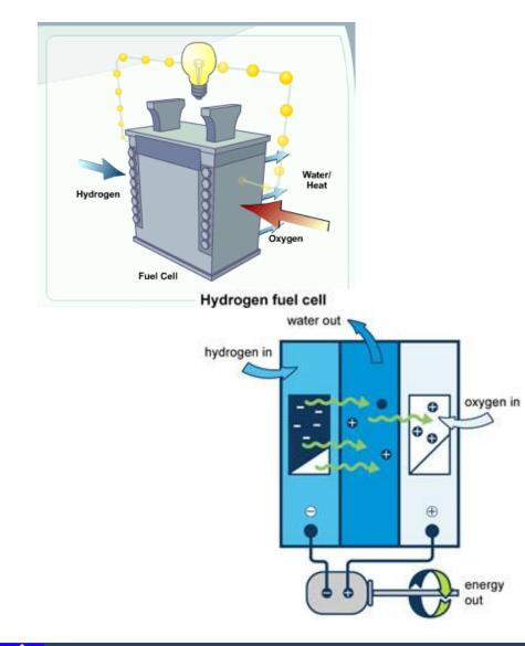
A fuel cell is a device that uses hydrogen (or hydrogen-rich fuel) and oxygen to create electricity. Fuel cells are more energy-efficient than combustion engines and the hydrogen used to power them can come from a variety of sources.
