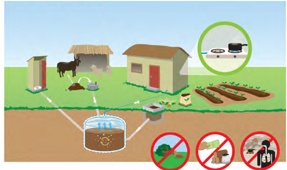
The Bio-Gas Digester:
