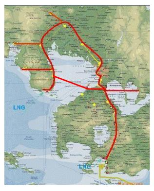
Figure 6. The identified critical pipeline infrastructure to expand the use of natural gas namely, the Batangas-Manila Pipeline (BatMan 1) and the Bataan-Manila Pipeline (BatMan 2) and a possible undersea Batangas-Cavite Pipeline (BatCave).
