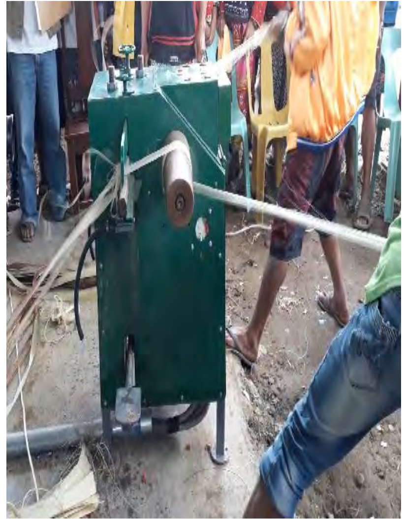
Abaca spindle machine
