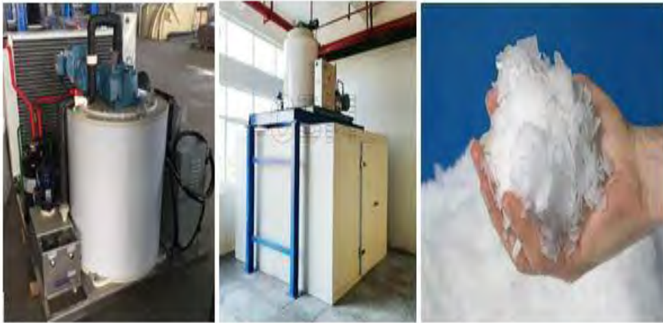
Proposed flake ice making system(left) and the product of flake ice (right)
