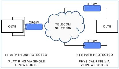
Following is an illustration of a non-protected versus ring or 1+1 protected optical network connection.
