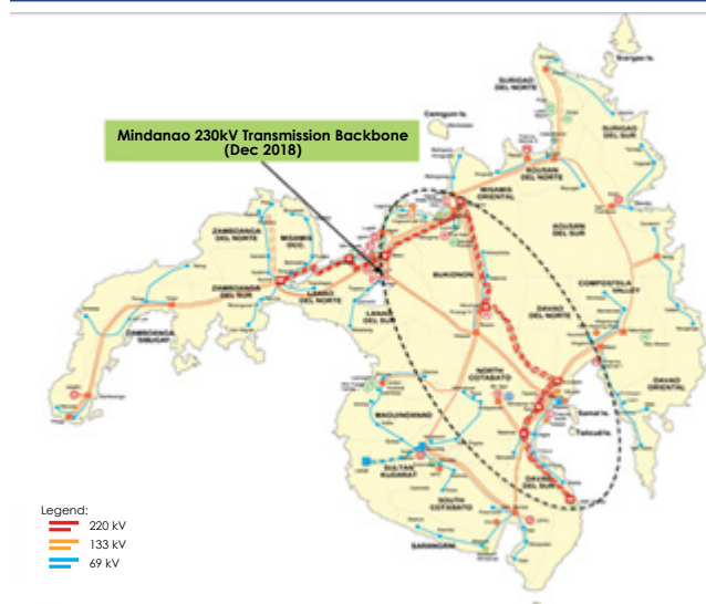
Figure 55. MINDANAO 230 kV TRANSMISSION BACKBONE
